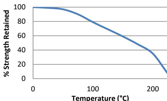
"Hot strength" shear strength tests performed on mild steel. Fully cured specimens conditioned to pull temperature for 30 minutes before testing at temperature. TA437 can withstand higher temperatures for brief periods (such as for paint baking and wave soldering processes) providing the joint is not unduly stressed. The minimum temperature the cured adhesive can be exposed to is -55°C (-65°F) depending on the materials being bonded.
