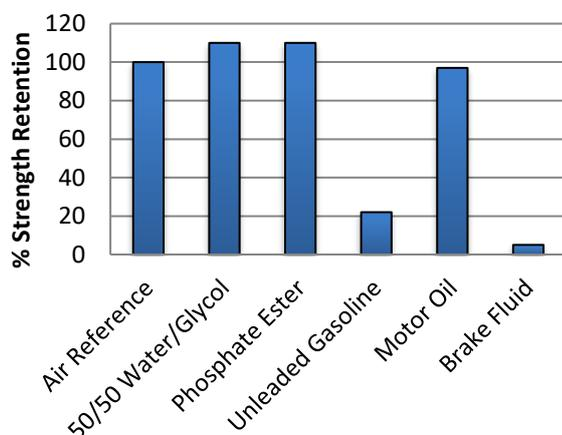
Specimens were immersed for 30 days at 85°C and tested at room temperature.
